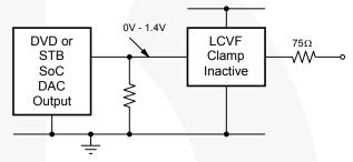
Figure 12.DC-Coupled Inputs and Outputs
