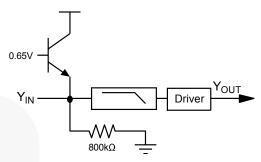
Figure 11. Input Clamp Circuit
