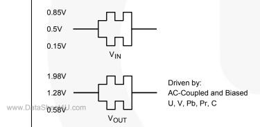
Figure 10. Typical Voltage Levels
