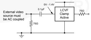
Figure 14.SCART Configuration with DC-Coupled Outputs
