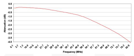
Figure 6. FMS6646 HD Frequency Response (Flatness)
