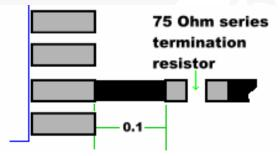
Figure 19. Distance from Device Pin to Series
