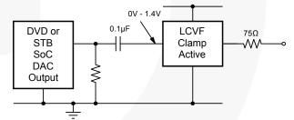
Figure 13.AC-Coupled Inputs, DC-Coupled Outputs
