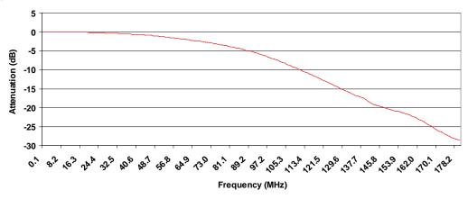
Figure 5. FMS6646 HD Frequency Response
