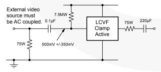
Figure 18. Biased SCART with AC-Coupled Outputs
