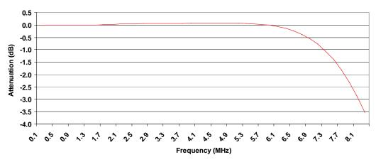
Figure 4. FMS6646 SD Frequency Response (Flatness)
