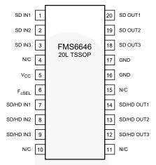
Figure 2. Pin Configuration
