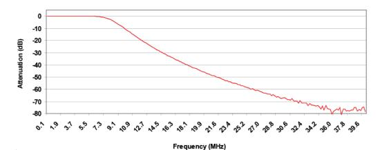
Figure 3. FMS6646 SD Frequency Response
