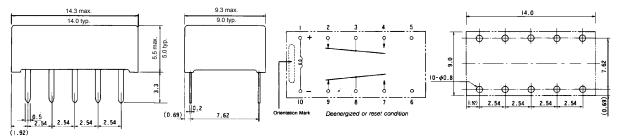
AL-D type (Double winding latching type)
