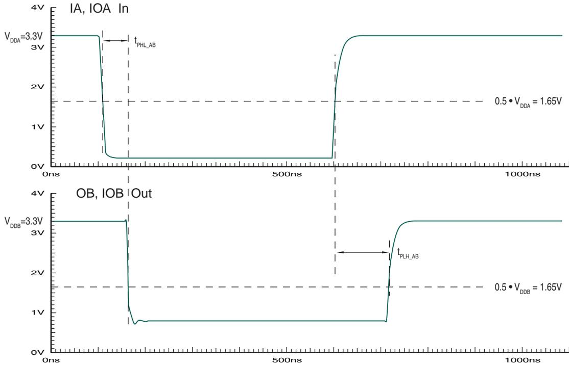
1.10 IOB to IOA Switching Waveforms
