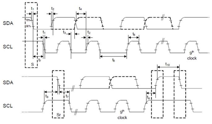
Figure 5 Standard I2C mode timing.
