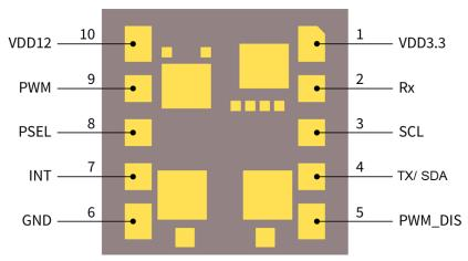
Figure 2 Pin-out diagram (Bottom view)
