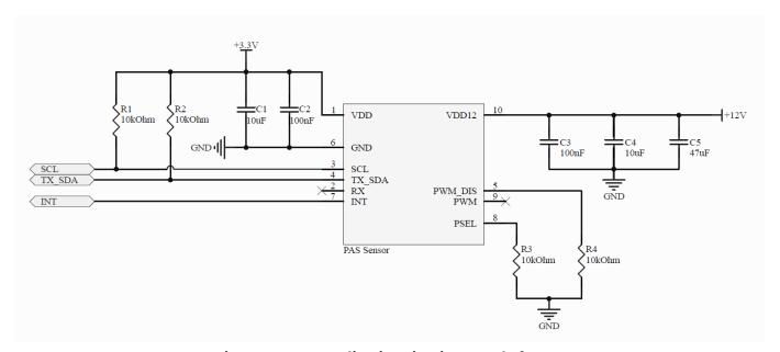
Figure 6 Application circuit example for I2C
