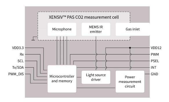
Figure 1 Block diagram of XENSIV™ PAS CO2
