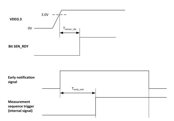
Figure 4 Illustration of the timing characteristic parameters
