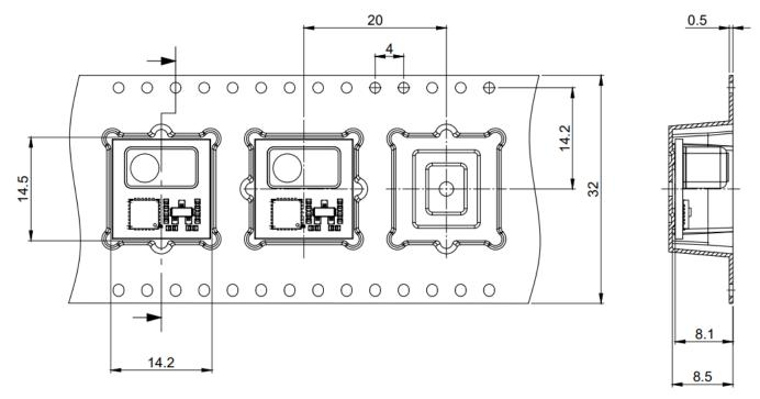
Figure 11 Tape and reel packing of XENSIV<sup>™</sup> PAS CO2
