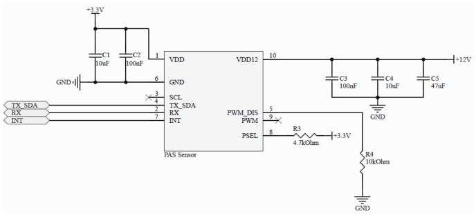
Figure 7 Application circuit example for UART
