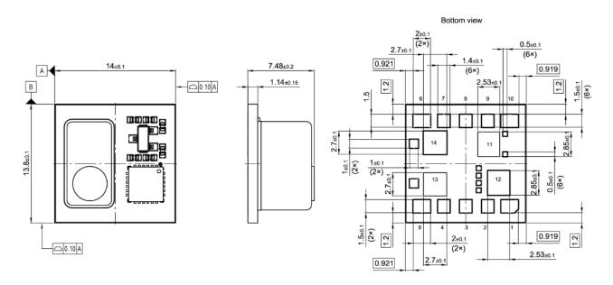
Figure 10 Package dimensions of XENSIV<sup>™</sup> PAS CO2.
