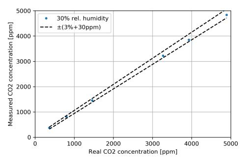
Figure 3 The typical sensor response to the CO<sub>2</sub> concentration change.
