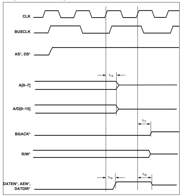
Figure 28. DMA Read Cycle Timing
