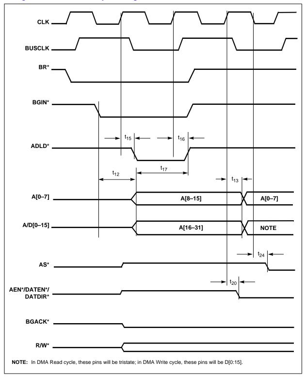
Figure 26. Bus Release Timing
