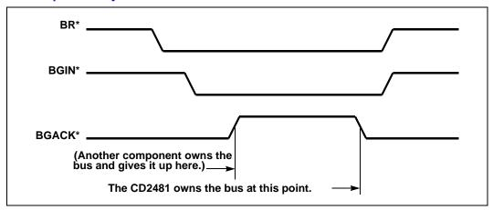
Figure 6. Data Transfer Timing
