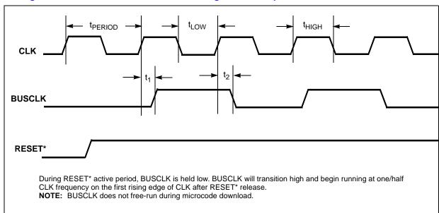
Figure 22. Slave Read Cycle Timing
