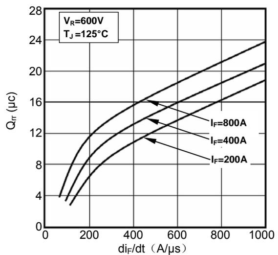
Figure4. Reverse Recovery Charge vs di<sub>F</sub>/dt
