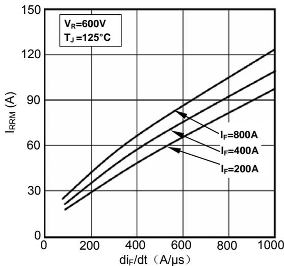
Figure3. Reverse Recovery Current vs di<sub>F</sub>/dt
