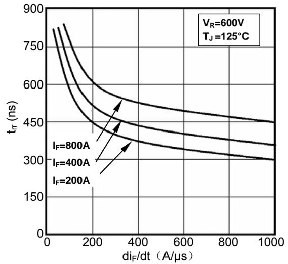
Figure2. Reverse Recovery Time vs di<sub>F</sub>/dt
