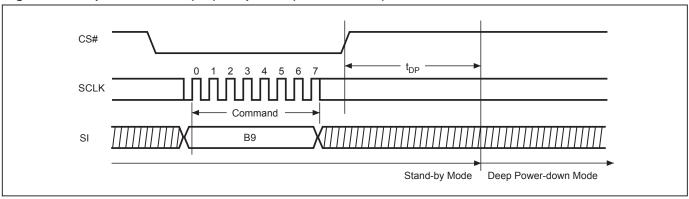
Figure 23. Release from Deep Power-down and Read Electronic Signature (RES) Sequence (Command AB)
