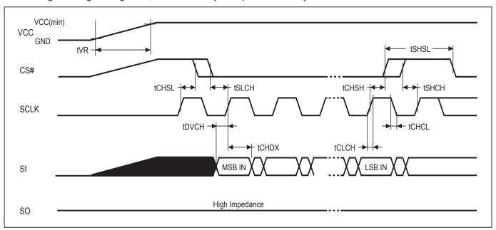
Figure A. AC Timing at Device Power-Up
