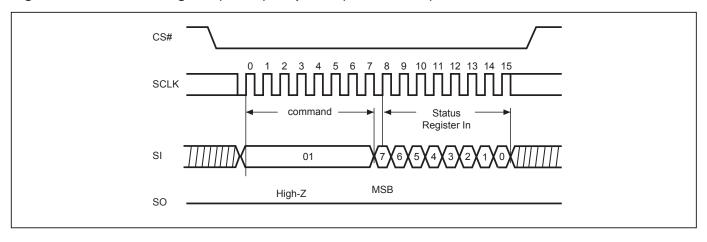
Figure 16. Read Data Bytes (READ) Sequence (Command 03)
