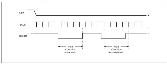
The Serial Data Output (SO) is high impedance, both Serial Data Input (SI) and Serial Clock (SCLK) are don't care during the HOLD operation. If Chip Select (CS#) drives high during HOLD operation, it will reset the internal logic of the device. To re-start communication with chip, the HOLD# must be at high and CS# must be at low.
