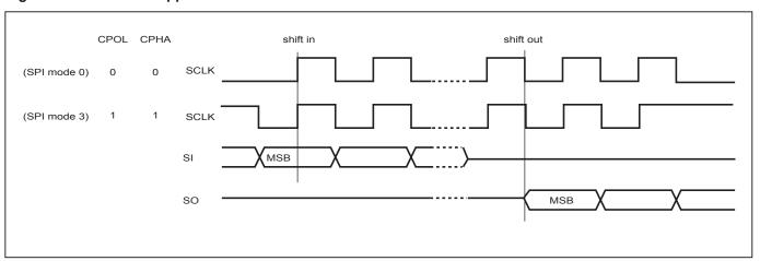
Figure 2. SPI Modes Supported
