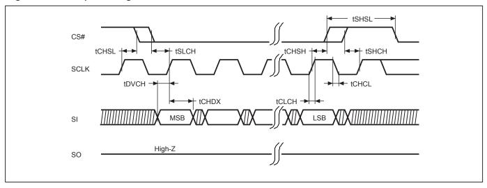
Figure 8. Output Timing
