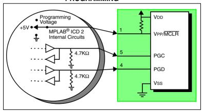
A simplified diagram of some of the internal interface circuitry of the MPLAB ICD 2 is shown. For programming, no clock is needed on the target PICmicro MCU, but power must be supplied. When programming, MPLAB ICD 2 puts programming levels on VPP, sends clock pulses on PGC and serial data via PGD. To verify that the part has been programmed correctly, clocks are sent to PGC and data is read back from PGD. This conforms to the ICSP<sup>TM</sup> protocol of the PICmicro MCU under development.
