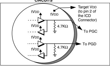
If MPLAB ICD 2 does not have voltage on its VDD line (pin 2 of the ICD connector) it will not operate. Using a scope, communications on PGC and PGD with a full target VDD to VSS peak-to-peak waveform should be seen. VPP should show +12, +5 and 0V levels depending upon the operation being performed. Signals should be seen on those lines only after performing an MPLAB ICD 2 function from the MPLAB user interface. Otherwise, all these lines should be idle and noise free.
