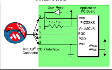
Although pin 2 (VDD) can supply a limited amount of power to the target application under certain conditions, for the purposes of these descriptions, pins 2 and 3 (VSS) are omitted. They are shown on the diagram for completeness, but in the following descriptions only three lines are active and relevant to core MPLAB ICD 2 operation: VPP/MCLR, PGC and PGD.
