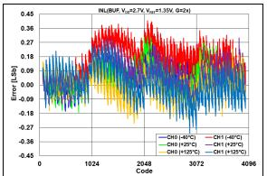
**FIGURE 2-52:** INL Error vs. DAC Code and Temperature,  $V_{DD} = 2.7V$ ,  $V_{REF} = 1.35V$ , G = 2x.
