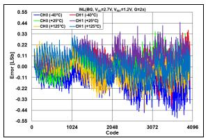
**FIGURE 2-40:** INL Error vs. DAC Code and Temperature,  $V_{DD} = 2.7V$ ,  $V_{REF} = 1.2V$ , G = 2x.
