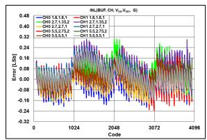
**FIGURE 2-53:** INL Error vs. DAC Code, Temperature = +25°C.
