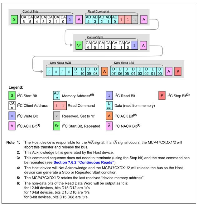
FIGURE 7-4: Read Command – Single Memory Address.
