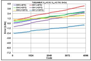
**FIGURE 2-23:** TUE ( $V_{OUT}$ ) vs. DAC Code and Temperature,  $V_{DD} = 5.5V$ ,  $V_{REF} = 2.75V$ , G = 2x.
