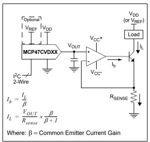
**FIGURE 8-8:** Digitally-Controlled Current Source.
