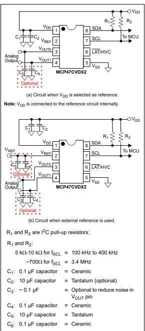
FIGURE 8-2: Example Circuit.
