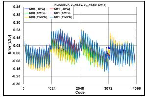
**FIGURE 2-42:** INL Error vs. DAC Code and Temperature,  $V_{DD} = V_{REF} = 5.5V$ , G = 1x.
