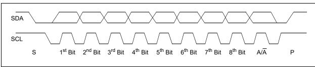
FIGURE B-7: Typical 8-Bit I<sup>2</sup>C Waveform Format.
