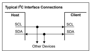
**FIGURE B-1:** Typical I<sup>2</sup>C Interface.
