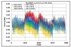
**FIGURE 2-46:** INL Error vs. DAC Code and Temperature,  $V_{DD} = 2.7V$ ,  $V_{REF} = 1.35V$ , G = 2x.
