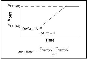
FIGURE 5-6: V<sub>OUT</sub> Pin Slew Rate.
