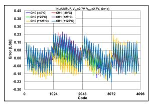
**FIGURE 2-43:** INL Error vs. DAC Code and Temperature,  $V_{DD} = V_{REF} = 2.7V$ , G = 1x.
