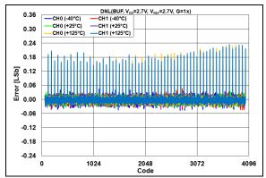
**FIGURE 2-71:** DNL Error vs. DAC Code and Temperature,  $V_{DD} = V_{REF} = 2.7V$ , G = 1x.
