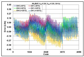
**FIGURE 2-50:** INL Error vs. DAC Code and Temperature,  $V_{DD} = V_{REF} = 1.8V$ , G = 1x.
