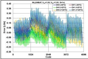
FIGURE 2-44: INL Error vs. DAC Code and Temperature,  $V_{DD} = V_{REF} = 1.8V$ , G = 1x.
