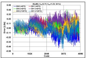
**FIGURE 2-37:** INL Error vs. DAC Code and Temperature,  $V_{DD} = 2.7V$ ,  $V_{REF} = 1.2V$ , G = 1x.
