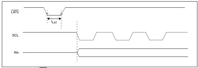
FIGURE 1-2: LAT Pin Waveforms.
