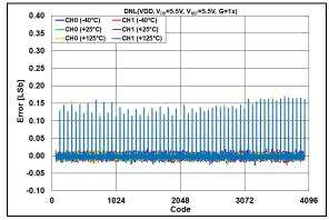
**FIGURE 2-54:** DNL Error vs. DAC Code and Temperature,  $V_{REF} = V_{DD} = 5.5V$ , G = 1x.
