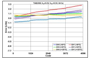
**FIGURE 2-10:** TUE ( $V_{OUT}$ ) vs. DAC Code and Temperature,  $V_{REF} = V_{DD} = 5.5V$ , G = 1x.
