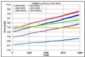
**FIGURE 2-14:** TUE  $(V_{OUT})$  vs. DAC Code and Temperature,  $V_{DD} = 5.5V$ ,  $V_{REF} = 1.2V$ , G = 1x.
