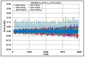
**FIGURE 2-73:** DNL Error vs. DAC Code and Temperature,  $V_{DD} = 5.5V$ ,  $V_{REF} = 2.75V$ , G = 1x.
