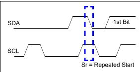
FIGURE B-5: Repeated Start Condition Waveform.
