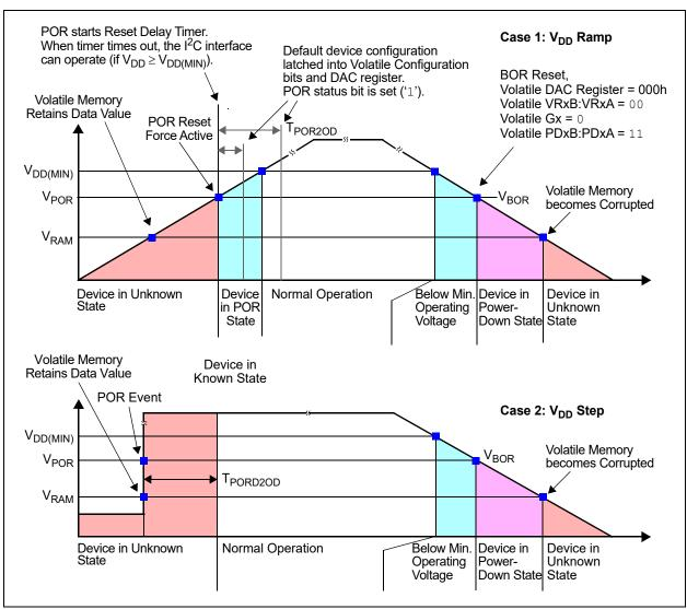
FIGURE 4-1: Power-on Reset Operation.
