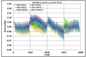
**FIGURE 2-32:** INL Error vs. DAC Code and Temperature,  $V_{REF} = V_{DD} = 5.5V$ , G = 1x.
