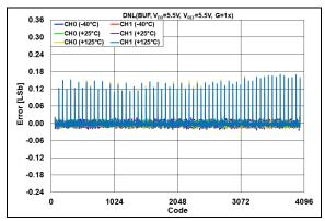
**FIGURE 2-70:** DNL Error vs. DAC Code and Temperature,  $V_{DD} = V_{REF} = 5.5V$ , G = 1x.
