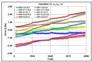
**FIGURE 2-25:** TUE  $(V_{OUT})$  vs. DAC Code, Temperature = +25°C.
