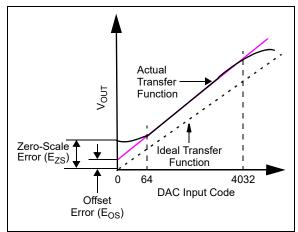
FIGURE C-2: Offset Error (Zero Gain Error).
