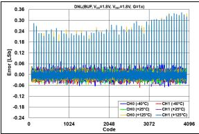
**FIGURE 2-72:** DNL Error vs. DAC Code and Temperature,  $V_{REF} = V_{DD} = 1.8V$ , G = 1x.
