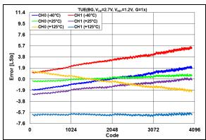
**FIGURE 2-15:** TUE  $(V_{OUT})$  vs. DAC Code and Temperature,  $V_{DD} = 2.7V$ ,  $V_{REF} = 1.2V$ , G = 1x.
