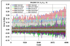
FIGURE 2-75: DNL Error vs. DAC Code, Temperature = +25°C.
