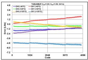
**FIGURE 2-22:** TUE  $(V_{OUT})$  vs. DAC Code and Temperature,  $V_{REF} = V_{DD} = 1.8V$ , G = 1x.
