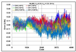
**FIGURE 2-36:** INL Error vs. DAC Code and Temperature,  $V_{DD} = 5.5V$ ,  $V_{REF} = 1.2V$ , G = 1x.
