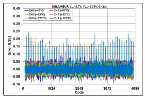
**FIGURE 2-68:** DNL Error vs. DAC Code and Temperature,  $V_{DD} = 2.7V$ ,  $V_{REF} = 1.35V$ , G = 2x.
