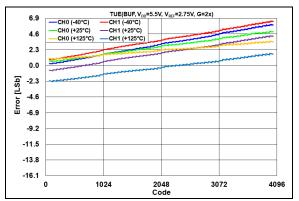
**FIGURE 2-29:** TUE ( $V_{OUT}$ ) vs. DAC Code and Temperature,  $V_{REF}$  = 2.75V,  $V_{DD}$  = 5.5V, G = 2x.
