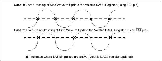
FIGURE 5-9: Example Use of LAT Pin Operation.
