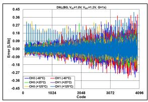
**FIGURE 2-60:** DNL Error vs. DAC Code and Temperature,  $V_{DD} = 1.8V$ ,  $V_{REF} = 1.2V$ , G = 1x.
