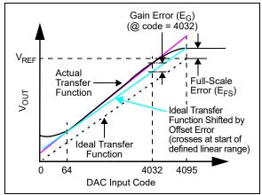
**FIGURE C-3:** Gain Error and Full-Scale Error Example.
