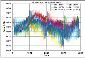
**FIGURE 2-34:** INL Error vs. DAC Code and Temperature,  $V_{REF} = V_{DD} = 1.8V$ , G = 1x.
