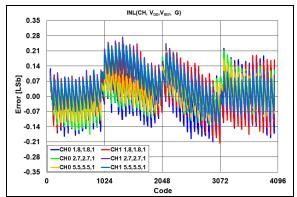
FIGURE 2-35: INL Error vs. DAC Code, Temperature = +25°C.
