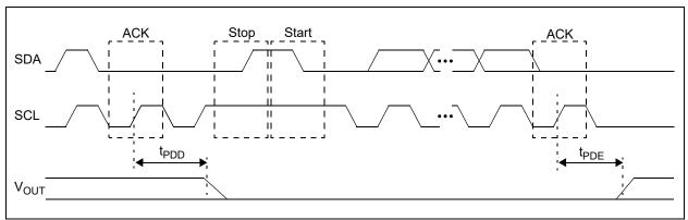
**FIGURE 1-4:** I<sup>2</sup>C Power-Down Command Timing.
