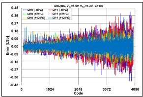
**FIGURE 2-58:** DNL Error vs. DAC Code and Temperature,  $V_{DD} = 5.5V$ ,  $V_{REF} = 1.2V$ , G = 1x.
