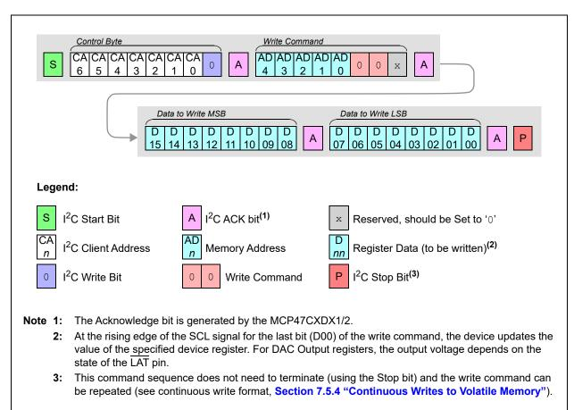
FIGURE 7-1: Write Random Address Command.
