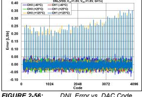
**FIGURE 2-56:** DNL Error vs. DAC Code and Temperature,  $V_{REF} = V_{DD} = 1.8V$ , G = 1x.
