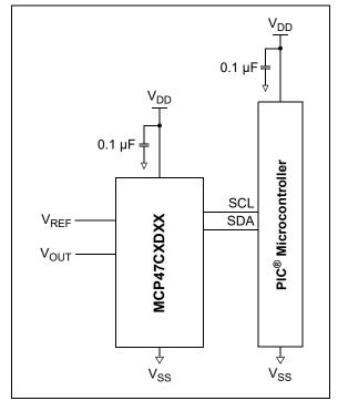
FIGURE 8-10: Typical Microcontroller Connections.
