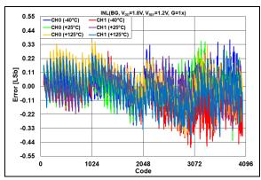
**FIGURE 2-38:** INL Error vs. DAC Code and Temperature,  $V_{DD} = 1.8V$ ,  $V_{REF} = 1.2V$ , G = 1x.
