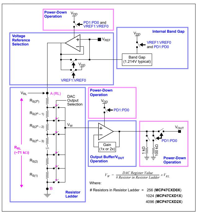
FIGURE 5-1: MCP47CXDX1/2 DAC Module Block Diagram.
