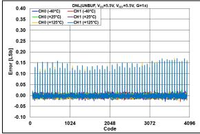
**FIGURE 2-64:** DNL Error vs. DAC Code and Temperature,  $V_{DD} = V_{REF} = 5.5V$ , G = 1x.
