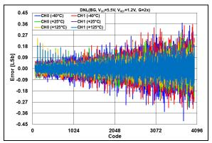
**FIGURE 2-61:** DNL Error vs. DAC Code and Temperature,  $V_{DD} = 5.5V$ ,  $V_{REF} = 1.2V$ , G = 2x.
