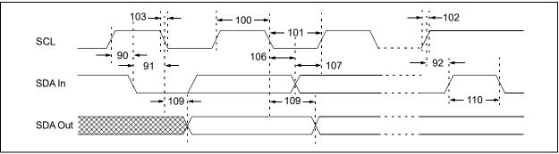
FIGURE 1-6: I<sup>2</sup>C Bus Data Timing Waveforms.
