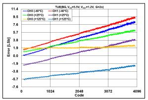
**FIGURE 2-17:** TUE  $(V_{OUT})$  vs. DAC Code and Temperature,  $V_{DD} = 5.5V$ ,  $V_{REF} = 1.2V$ , G = 2x.
