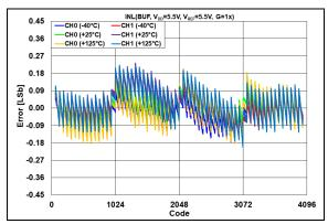
**FIGURE 2-48:** INL Error vs. DAC Code and Temperature,  $V_{DD} = V_{REF} = 5.5V$ , G = 1x.
