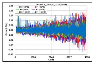
**FIGURE 2-62:** DNL Error vs. DAC Code and Temperature,  $V_{DD} = 2.7V$ ,  $V_{REF} = 1.2V$ , G = 2x.
