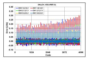
**FIGURE 2-57:** DNL Error vs. DAC Code, Temperature = +25°C.
