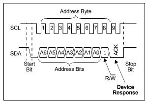
FIGURE 8-1: I<sup>2</sup>C Bus Connection Test.
