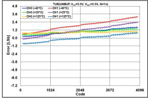
**FIGURE 2-20:** TUE  $(V_{OUT})$  vs. DAC Code and Temperature,  $V_{REF} = V_{DD} = 5.5V$ , G = 1x.
