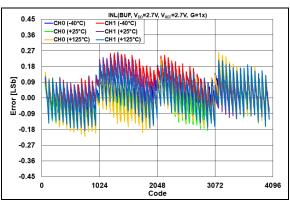
**FIGURE 2-49:** INL Error vs. DAC Code and Temperature,  $V_{DD} = V_{REF} = 2.7V$ , G = 1x.
