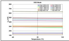
**FIGURE 2-1:** Average Device Supply Current vs.  $F_{SCL}$ , Voltage and Temperature – Active Interface, VRxB:VRxA = 00 (V<sub>DD</sub> Mode).
