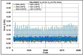
**FIGURE 2-67:** DNL Error vs. DAC Code and Temperature,  $V_{DD} = 5.5V$ ,  $V_{REF} = 2.75V$ , G = 2x.
