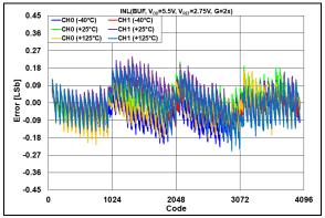
**FIGURE 2-51:** INL Error vs. DAC Code and Temperature,  $V_{DD} = 5.5V$ ,  $V_{REF} = 2.75V$ , G = 2x.
