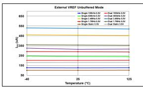
**FIGURE 2-3:** Average Device Supply Current vs.  $F_{SCL}$ , Voltage and Temperature – Active Interface, VRxB:VRxA = 10 (V<sub>REF</sub> Unbuffered Mode).
