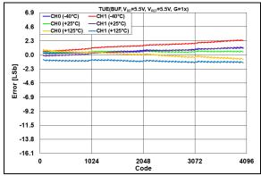
**FIGURE 2-26:** TUE  $(V_{OUT})$  vs. DAC Code and Temperature,  $V_{REF} = V_{DD} = 5.5V$ , G = 1x.
