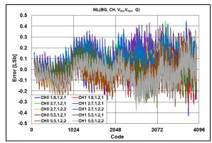
FIGURE 2-41: INL Error vs. DAC Code, Temperature = +25°C.
