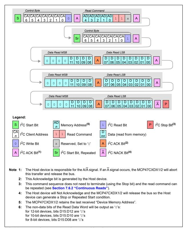
FIGURE 7-7: Continuous Read Command of Specified Address.
