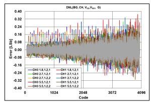
FIGURE 2-63: DNL Error vs. DAC Code, Temperature = +25°C.
