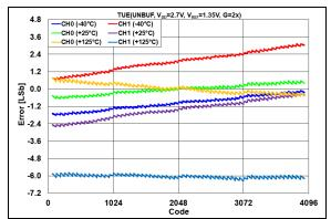
**FIGURE 2-24:** TUE  $(V_{OUT})$  vs. DAC Code and Temperature,  $V_{DD}$  = 2.7V,  $V_{REF}$  = 1.35V, G = 2x.
