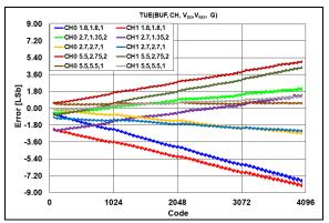
**FIGURE 2-31:** TUE  $(V_{OUT})$  vs. DAC Code, Temperature =  $+25^{\circ}$ C.
