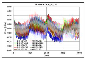
FIGURE 2-47: INL Error vs. DAC Code, Temperature = +25°C.
