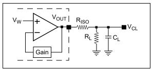
**FIGURE 5-7:** Circuit to Stabilize Output Buffer for Large Capacitive Loads  $(C_L)$ .
