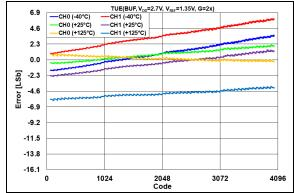
**FIGURE 2-30:** TUE  $(V_{OUT})$  vs. DAC Code and Temperature,  $V_{REF} = 1.35V$ ,  $V_{DD} = 2.7V$ , G = 2x.
