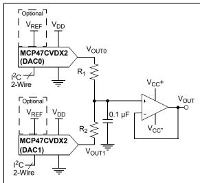
FIGURE 8-7: Simple Double Precision DAC Using MCP47CVDX2.
