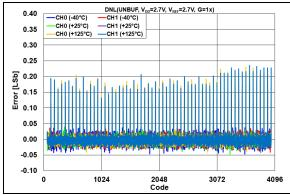
**FIGURE 2-65:** DNL Error vs. DAC Code and Temperature,  $V_{DD} = V_{REF} = 2.7V$ , G = 1x.
