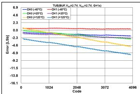
**FIGURE 2-27:** TUE  $(V_{OUT})$  vs. DAC Code and Temperature,  $V_{REF} = V_{DD} = 2.7V$ , G = 1x.
