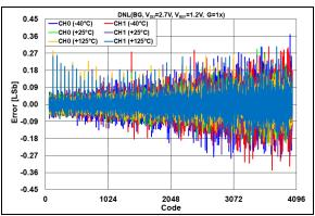
**FIGURE 2-59:** DNL Error vs. DAC Code and Temperature,  $V_{DD} = 2.7V$ ,  $V_{REF} = 1.2V$ , G = 1x.
