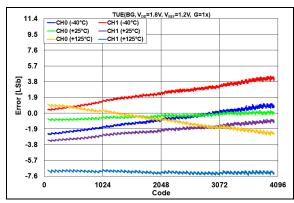
**FIGURE 2-16:** TUE  $(V_{OUT})$  vs. DAC Code and Temperature,  $V_{DD} = 1.8V$ ,  $V_{REF} = 1.2V$ , G = 1x.
