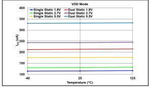
FIGURE 2-4: Average Device Supply Current vs. Voltage and Temperature – Inactive Interface, VRxB:VRxA = 00 (V<sub>DD</sub> Mode).
