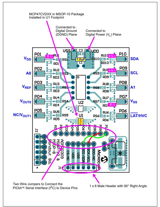
FIGURE 9-1: MCP47CXDX1/2 Evaluation Board Circuit Using ADM00309.
