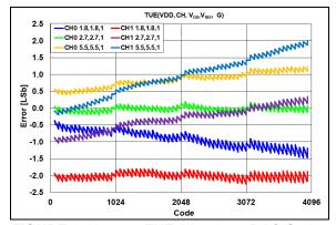
**FIGURE 2-13:** TUE  $(V_{OUT})$  vs. DAC Code, Temperature = +25°C.
