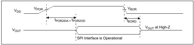
FIGURE 1-3: Power-on and Brown-out Reset Waveforms.
