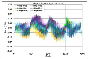
**FIGURE 2-33:** INL Error vs. DAC Code and Temperature,  $V_{REF} = V_{DD} = 2.7V$ , G = 1x.
