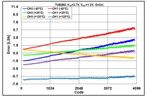
**FIGURE 2-18:** TUE  $(V_{OUT})$  vs. DAC Code and Temperature,  $V_{DD}$  = 2.7V,  $V_{REF}$  = 1.2V, G = 2x.
