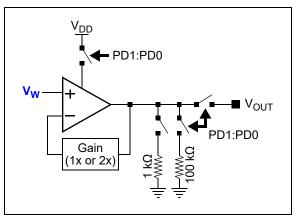
FIGURE 5-5: Output Driver Block Diagram.
