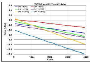
**FIGURE 2-28:** TUE  $(V_{OUT})$  vs. DAC Code and Temperature,  $V_{REF} = V_{DD} = 2.7V$ , G = 1x.
