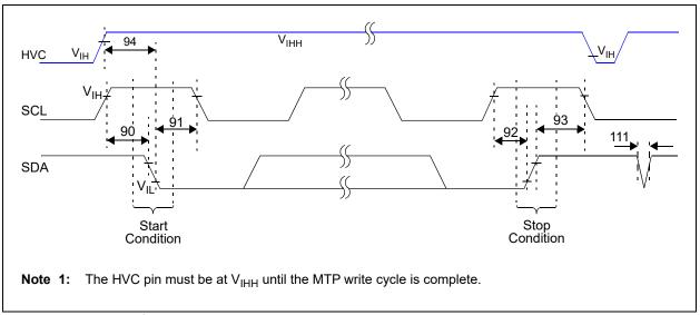
FIGURE 1-5: I<sup>2</sup>C Bus Start/Stop Bits and HVC Timing Waveforms.
