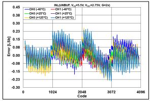
FIGURE 2-45: INL Error vs. DAC Code and Temperature,  $V_{DD} = 5.5V$ ,  $V_{REF} = 2.75V$ , G = 2x.
