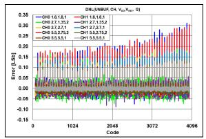
**FIGURE 2-69:** DNL Error vs. DAC Code, Temperature = +25°C.
