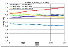
**FIGURE 2-11:** TUE  $(V_{OUT})$  vs. DAC Code and Temperature,  $V_{REF} = V_{DD} = 2.7V$ , G = 1x.
