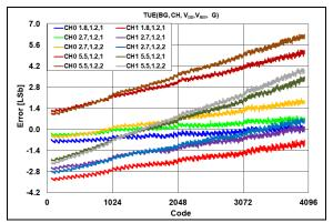
**FIGURE 2-19:** TUE  $(V_{OUT})$  vs. DAC Code, Temperature = +25°C.
