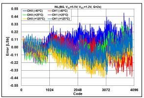
**FIGURE 2-39:** INL Error vs. DAC Code and Temperature,  $V_{DD} = 5.5V$ ,  $V_{REF} = 1.2V$ , G = 2x.
