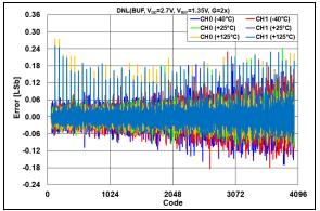
**FIGURE 2-74:** DNL Error vs. DAC Code and Temperature,  $V_{DD} = 2.7V$ ,  $V_{REF} = 1.35V$ , G = 2x.
