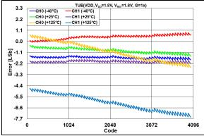
**FIGURE 2-12:** TUE  $(V_{OUT})$  vs. DAC Code and Temperature,  $V_{REF} = V_{DD} = 1.8V$ , G = 1x.
