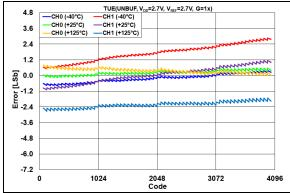
**FIGURE 2-21:** TUE  $(V_{OUT})$  vs. DAC Code and Temperature,  $V_{REF} = V_{DD} = 2.7V$ , G = 1x.
