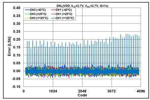
**FIGURE 2-55:** DNL Error vs. DAC Code and Temperature,  $V_{REF} = V_{DD} = 2.7V$ , G = 1x.
