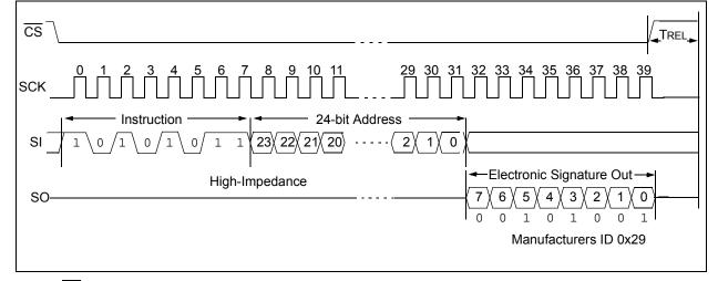
Driving  $\overline{CS}$  high after the 8-bit RDID command, but before the electronic signature has been transmitted, will still ensure the device will be taken out of Deep Power-Down mode, as shown in Figure 2-13.
