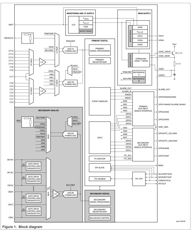
14 cells battery cell controller IC
