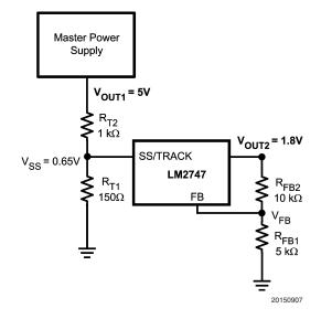
FIGURE 3. Tracking Circuit
