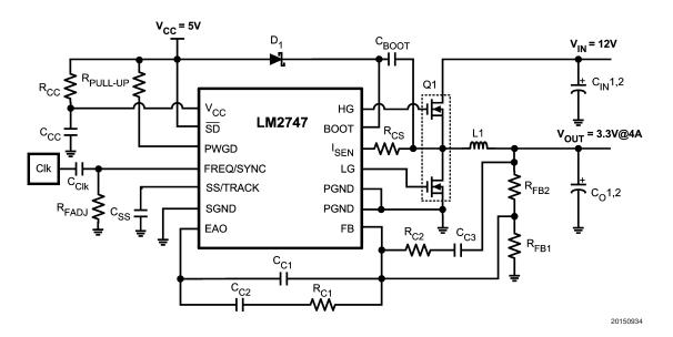
FIGURE 19. 12V to 3.3V @ 4A,  $f_{SW}$  = 300kHz
