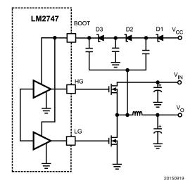
FIGURE 11. Charge Pump with Added Gate Drive
