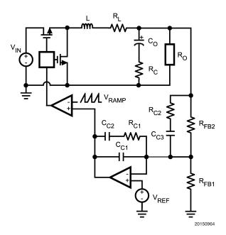
FIGURE 13. Power Stage and Error Amp
