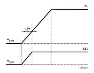
FIGURE 5. Tracking with Equal Slew Rates
