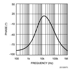
FIGURE 15. Error Amp. Gain and Phase
