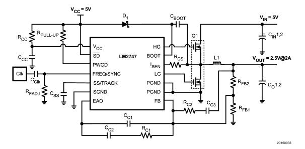
FIGURE 18. 5V to 2.5V @ 2A,  $f_{SW}$  = 300 kHz
