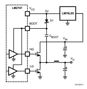
FIGURE 10. LM78L05 Feeding Basic Charge Pump
