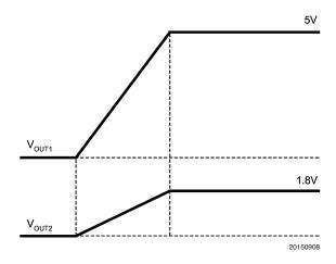
FIGURE 4. Tracking with Equal Soft-Start Time
