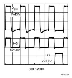
FIGURE 2. Output Pre-Bias Mode Waveforms
