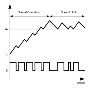
FIGURE 12. Current Limit Threshold
