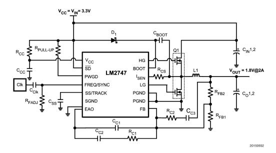
FIGURE 17. 3.3V to 1.8V @ 2A,  $f_{\text{SW}}$  = 300 kHz
