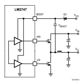
FIGURE 9. Basic Charge Pump (Bootstrap)
