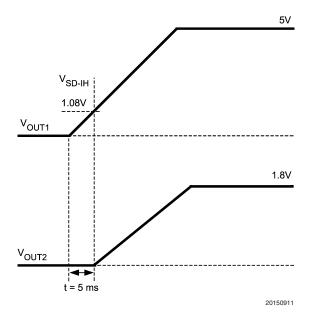
FIGURE 7. Delay for Sequencing
