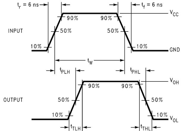
Figure 6. AC Waveforms
