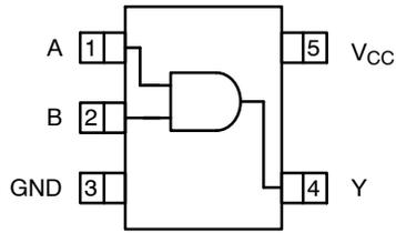
Figure 2. SOT23-5, SC-88A and SC-74A (Top View)
