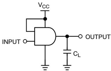
C<sub>L</sub> includes load and stray capacitance
