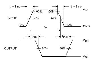
Figure 5. AC Waveforms
