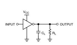
Figure 4. AC Test Circuit
