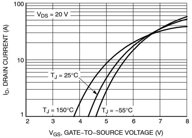
Figure 2. Transfer Characteristics
