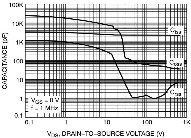
Figure 5. Capacitance Characteristics
