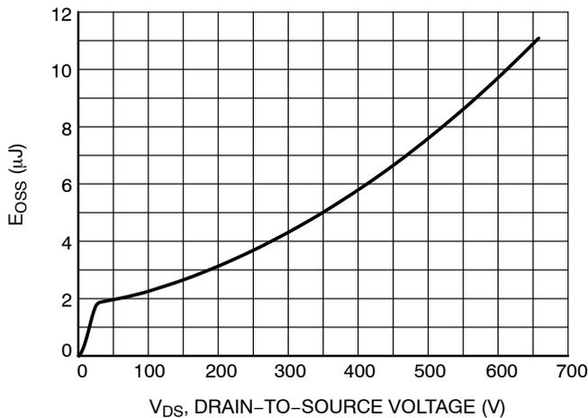
**Figure 11. E<sub>OSS</sub> vs. Drain-to-Source Voltage**
