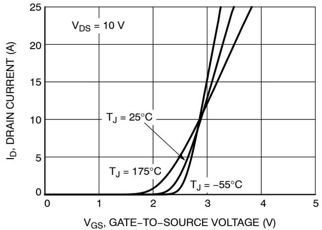
Figure 2. Transfer Characteristics
