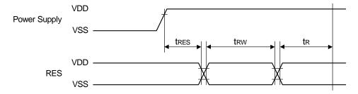
All signal timings are based on 20% and 80% of VDD signals.
