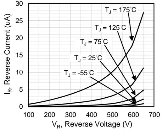
Fig.2 Reverse Characteristics
