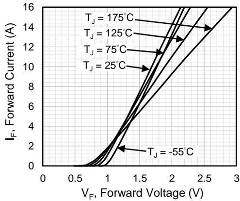
Fig.1 Forward Characteristics
