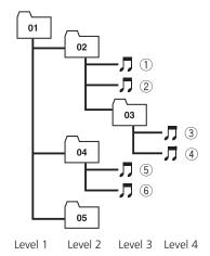
01 to 05 represent assigned folder numbers. ① to ⑥ represent the playback sequence. The user cannot assign folder numbers and specify the playback sequence with this unit.
