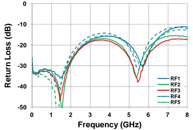
RFX Terminated Return Loss vs. Temperature
