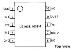
Note: both ground pins must be grounded.
