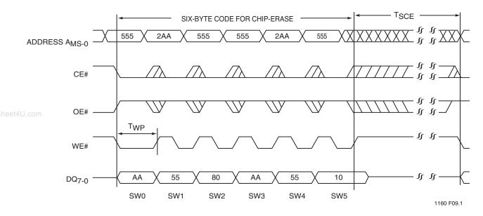
Note: This device also supports CE# controlled Chip-Erase operation The WE# and CE# signals are interchangeable as
