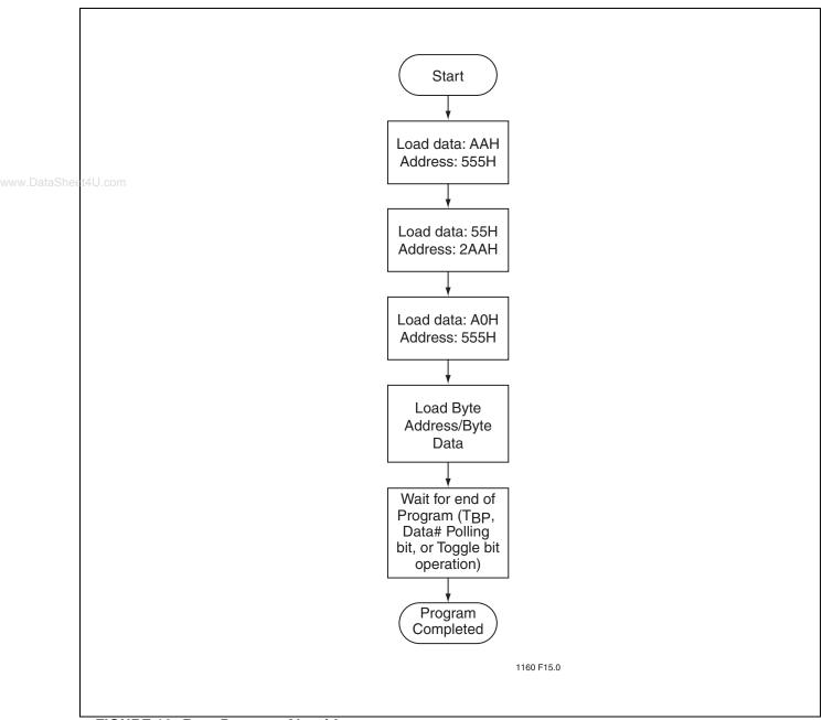
FIGURE 16: Byte-Program Algorithm
