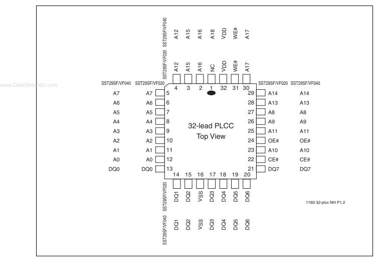
FIGURE 2: Pin Assignments for 32-lead PLCC
