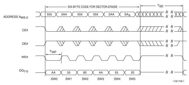
Note: This device also supports CE# controlled Sector-Erase operation The WE# and CE# signals are interchangeable as long as minimum timings are met. (See Table 11)
