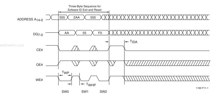
FIGURE 12: SOFTWARE ID EXIT AND RESET
