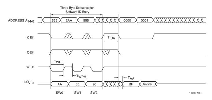
**Note:** Device ID = 24H for SST29SF020, 13H for SST29SF040 25H for SST29VF020, 14H for SST29VF040
