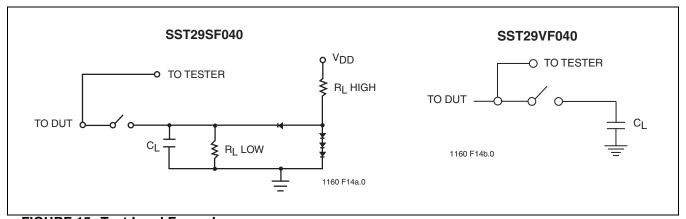
FIGURE 15: Test Load Examples
