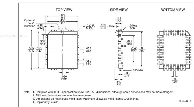
32-lead Plastic Lead Chip Carrier (PLCC)
