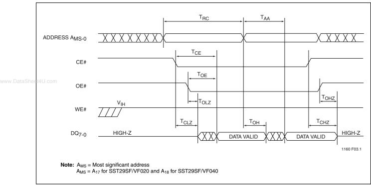
FIGURE 4: Read Cycle Timing Diagram
