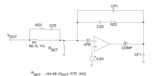
Type III Error Amplifier Compensation Circuit
