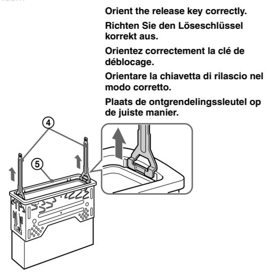
Orient the release key correctly.
