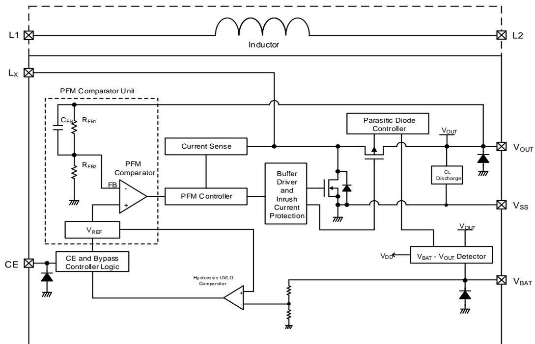
\* Diodes inside the circuits are ESD protection diodes and parasitic diodes.
