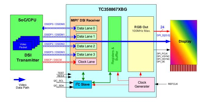
Figure 1.3 System Overview with TC358867XBG in MODE\_S2P Configuration
