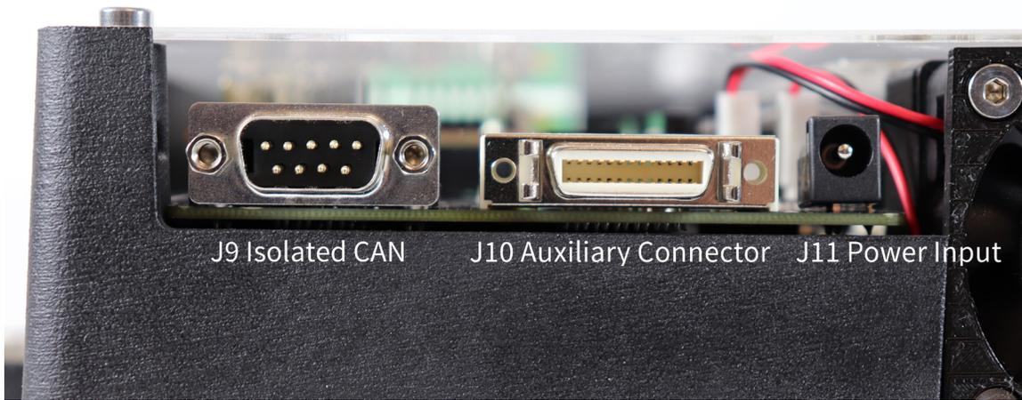
J9 Isolated CAN      J10 Auxiliary Connector      J11 Power Input
