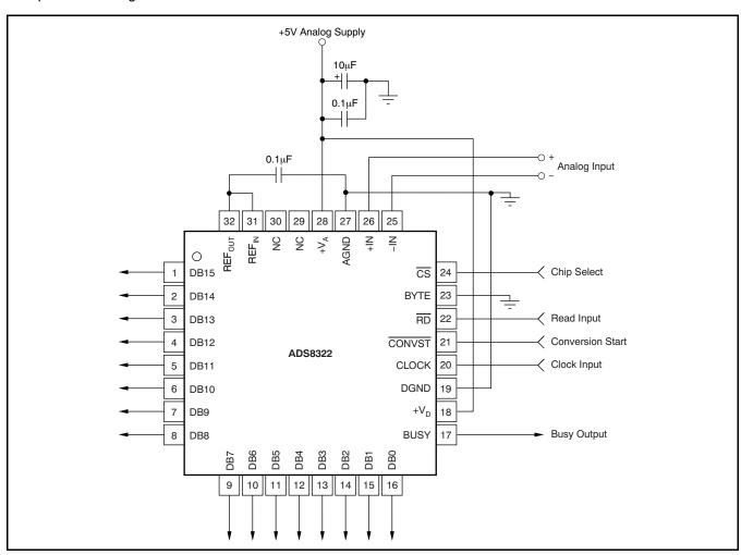
Figure 13. Typical Circuit Configuration
