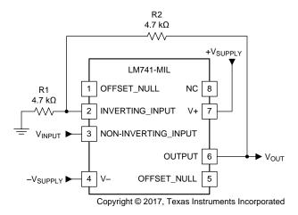
Figure 1. LM741-MIL Noninverting Amplifier Circuit
