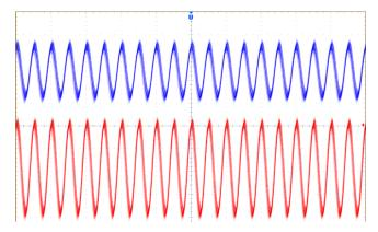
Figure 2. Waveforms for LM741-MIL Non-inverting Amplifier Circuit
