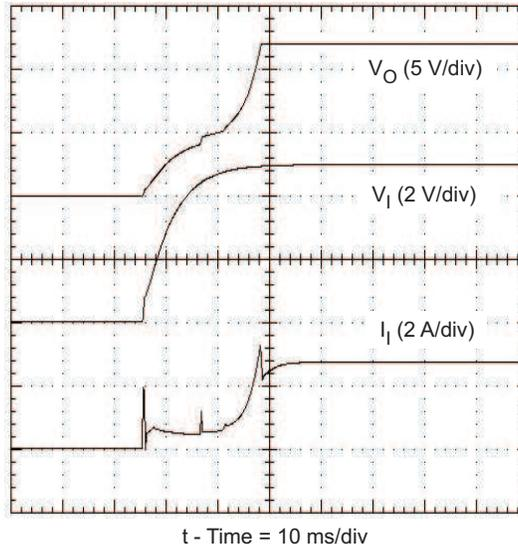
**Figure 15. Power-Up Waveforms**
