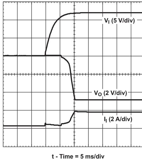
**Figure 19. Power-Up Waveforms**
