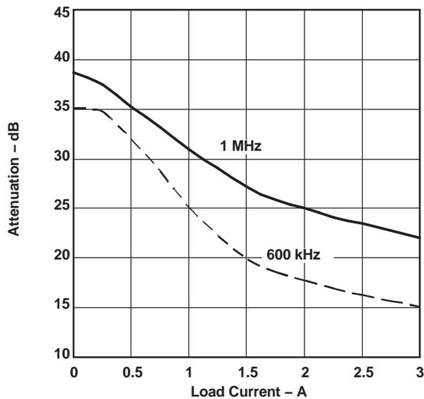
Figure 22.  $\pi$ -Filter Attenuation vs. Load Current
