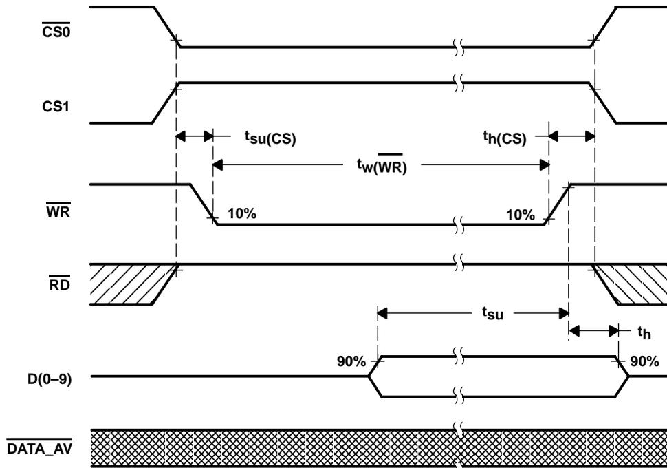
**Figure 30. Write Timing Diagram Using  $\overline{WR}$  ( $\overline{WR}$ -controlled)**
