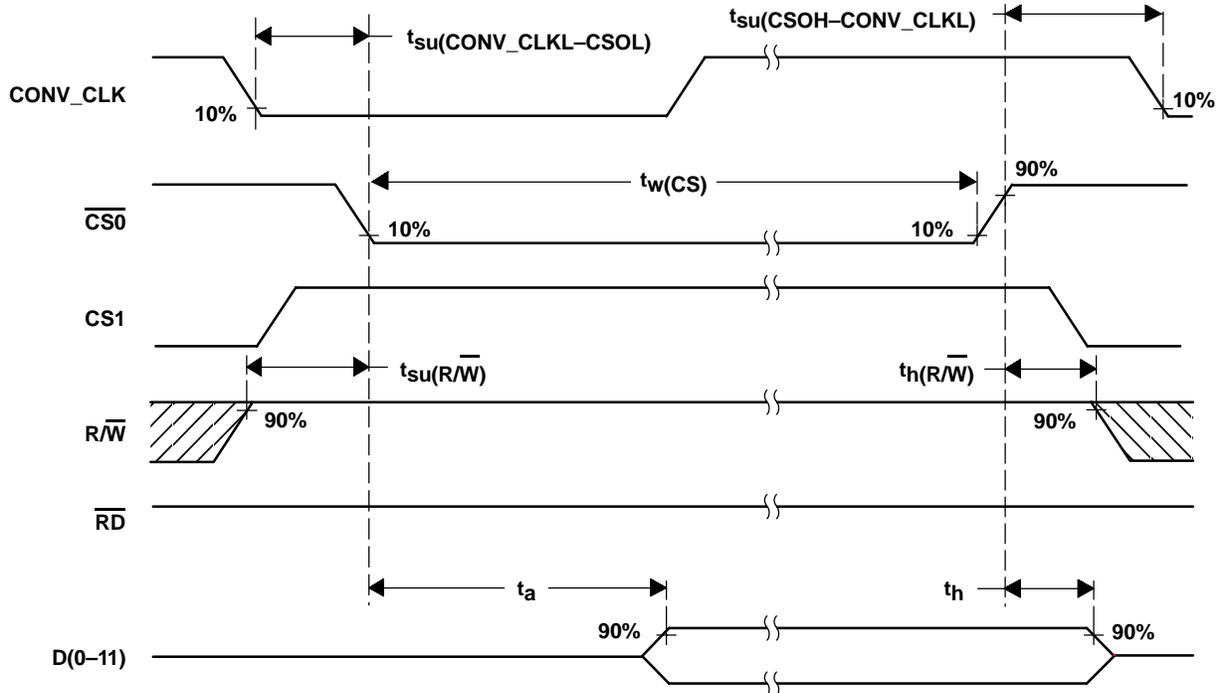
**Figure 31. Read Timing Diagram Using  $\overline{R/W}$  ( $\overline{CS0}$ -controlled)**
