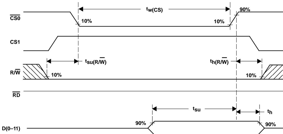
Figure 32. Write Timing Diagram Using  $\overline{R/\overline{W}}$  ( $\overline{CS0}$ -controlled)
