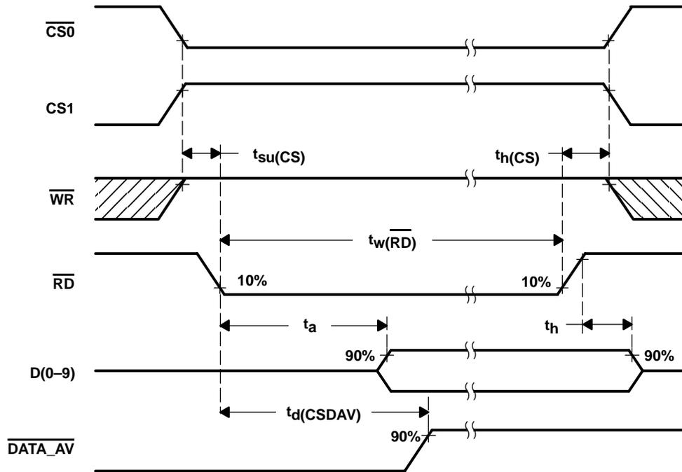
Figure 29. Read Timing Diagram Using  $\overline{RD}$  ( $\overline{RD}$ -controlled)
