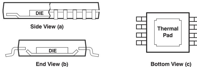
**Figure 47. Views of Thermally Enhanced DGN Package**
