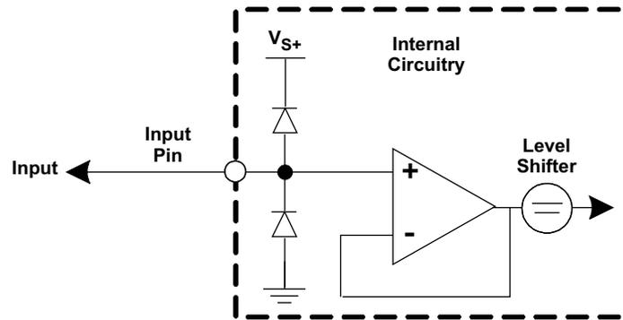
Figure 49. Equivalent DC + 135 mV Input Mode Circuit
