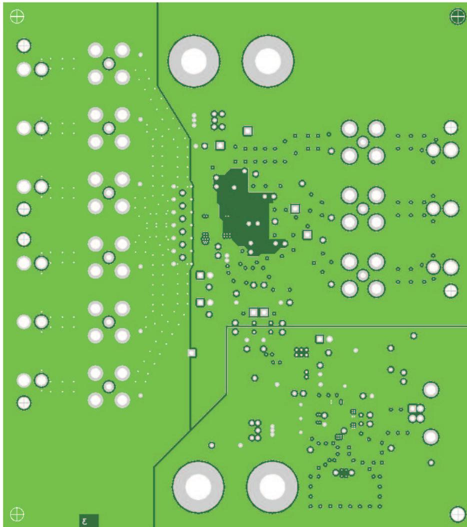
Figure 68. Layer Three - Power and Ground Layer
