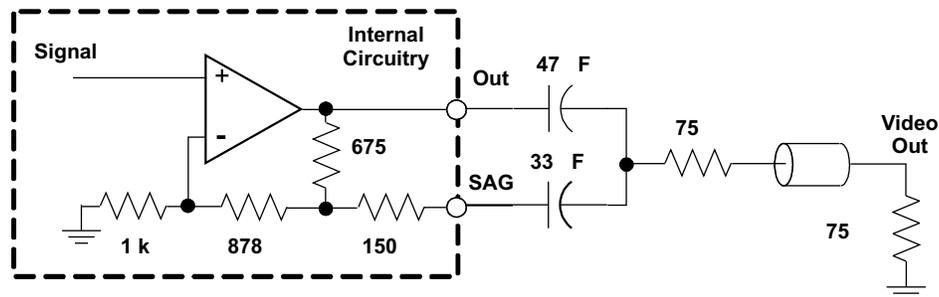
Figure 54. THS7313 Output Buffer Using SAG Corrected AC-Coupling
