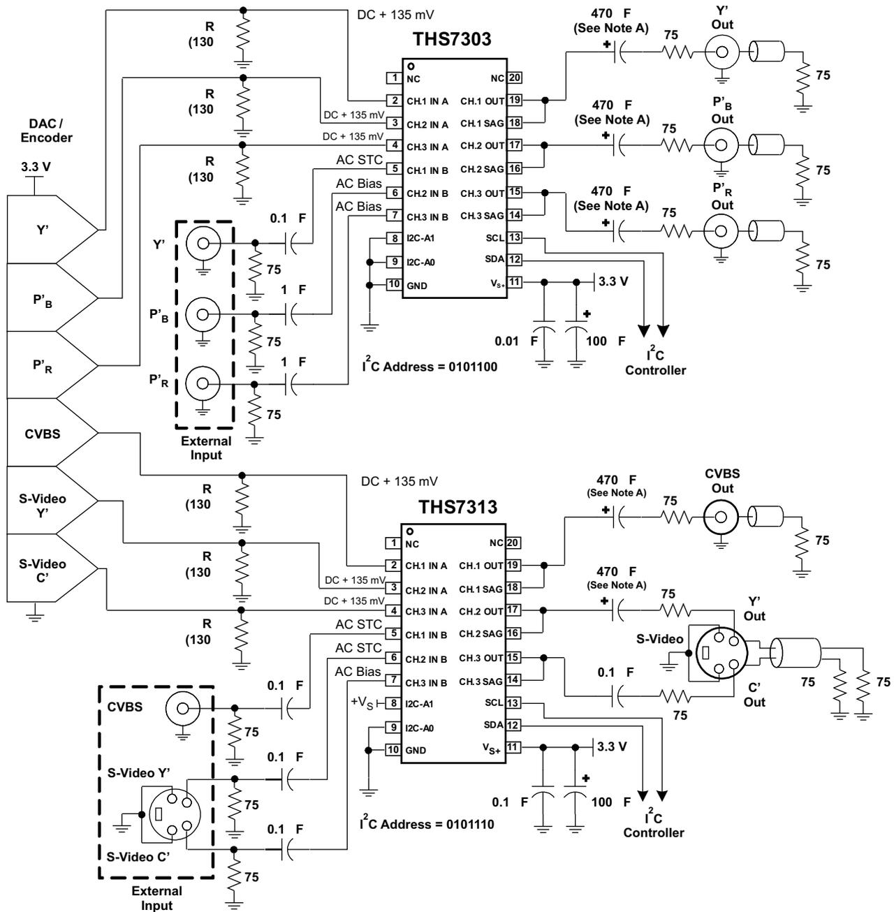
A. Due to the high frequency content of the video signal, it is recommended, but not required, to add a 0.01- $\mu$ F capacitor in parallel with these large capacitors.
