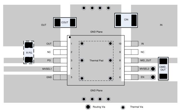
Figure 10-2. Fixed Version Layout Example
