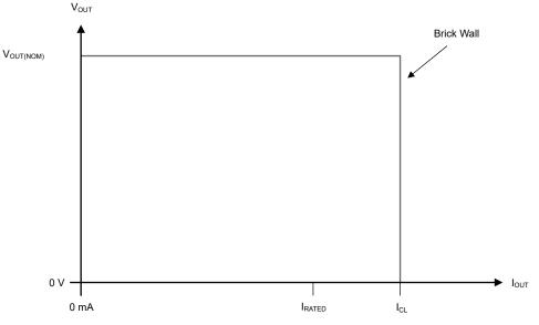
Figure 7-4. Current Limit: Brick-Wall Scheme
