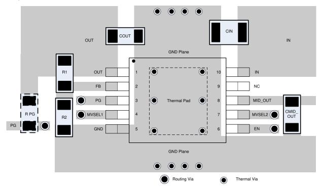
Figure 10-1. Adjustable Version Layout Example
