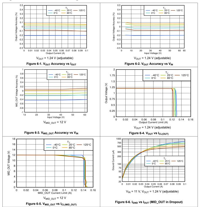
at operating temperature  $T_J = 25^{\circ}$ C,  $I_{OUT} = 1$  mA,  $I_{MID_OUT} = 0$  mA,  $V_{EN} = 2$  V,  $V_{MVSEL1} = 0.9$  V,  $V_{MVSEL2} = 0.9$  V,  $C_{IN} = 1 \mu$ F,  $C_{MID_OUT} = 4.7 \mu$ F,  $C_{OUT} = 1 \mu$ F, and  $V_{IN} = V_{MID_OUT} + 1.5$  V (unless otherwise noted); typical values are at  $T_J = 25^{\circ}$ C
