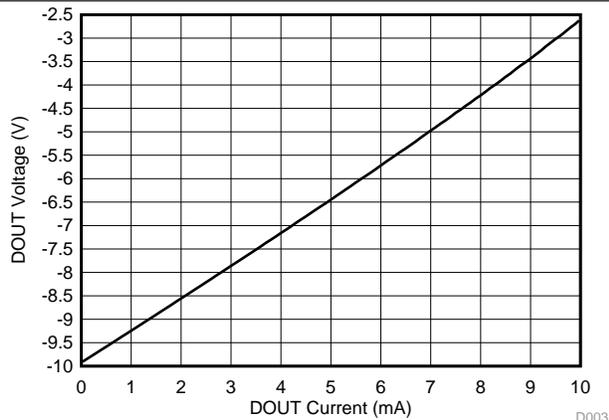
**Figure 3. Driver V<sub>OL</sub> vs Output Current**
