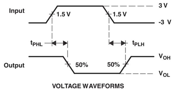
A. CL includes probe and jig capacitance.
