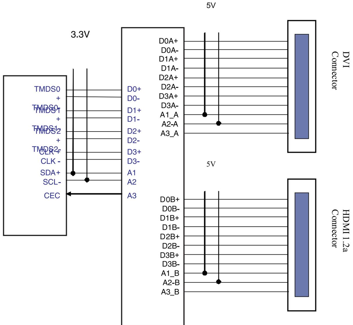
Figure 5. Typical Application Switching HDMI 1.2a and DVI
