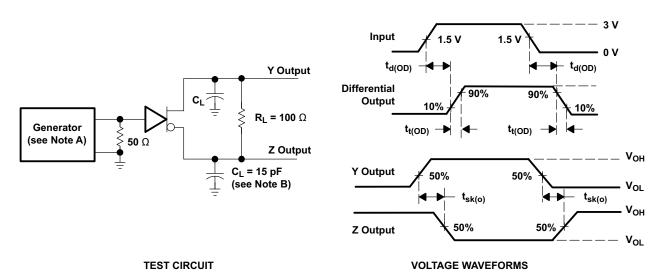
A. The input pulse generator has the following characteristics:  $Z_O = 50 \Omega$ , PRR  $\leq 500 \text{ kHz}$ ,  $t_w = 100 \text{ ns}$ ,  $t_r = \leq 5 \text{ ns}$ .
