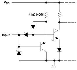
Figure 3. Equivalent of Each Input
