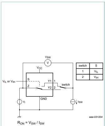
Fig. 6. Test circuit for measuring ON resistance
