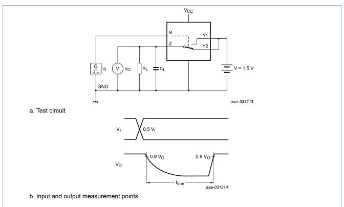
Fig. 15. Test circuit for measuring break-before-make times
