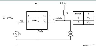
Adjust  $f_i$  voltage to obtain 0 dBm level at output. Increase  $f_i$  frequency until dB meter reads -3 dB.  $R_S = R_L = 50~\Omega$  (standard  $50~\Omega$  system).
