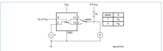
Fig. 17. Test circuit for measuring total harmonic distortion
