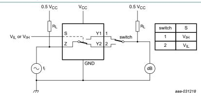
Adjust f<sub>i</sub> voltage to obtain 0 dBm level at input.
